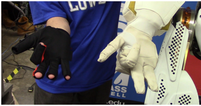
Figure 8: Manus VR Glove being used to control the robot's fingers in a direct 1-to-1 mode.
